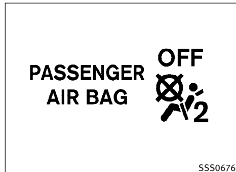
Front passenger air bag status light
